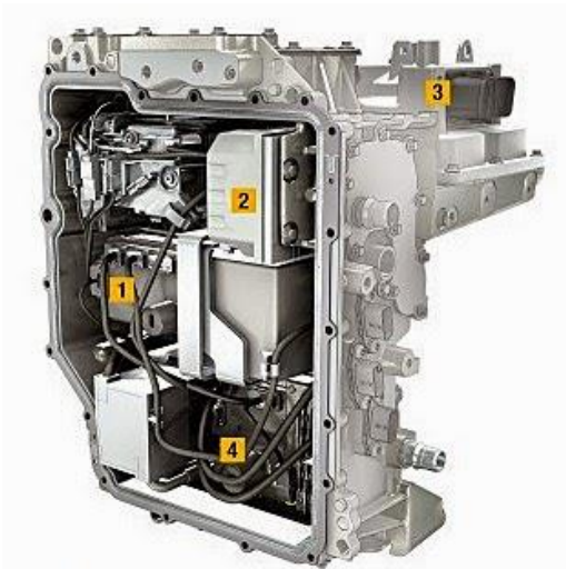
Power Electric Controler (PEC)
